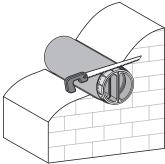
**9.** Install the sectional air flow separators from the outside
