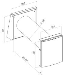
Overall dimensions of the indoor assembly unit  $[\mbox{\sc mm}]$
