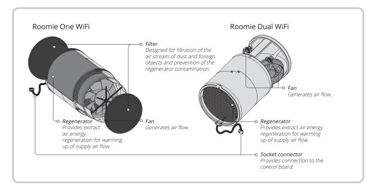
Cartridge is a solid block and cannot be dismantled. Roomie One WiFi has a cartridge with removable filters. They are removed for maintenance needs. A socket connector to be connected to the control board in the back part of the indoor unit is routed from the cartridge.
