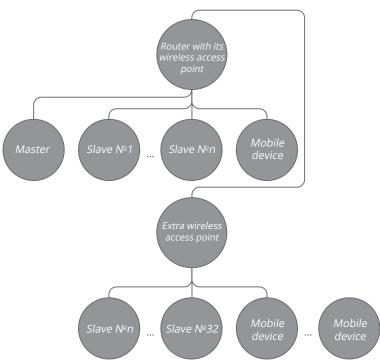
If the WiFi router capacity is not enough to connect a required number of the units, you may use an extra wireless access point to connect the other the unit. Optionally connection of several Master units to the network for arranging a zone control is also possible.
