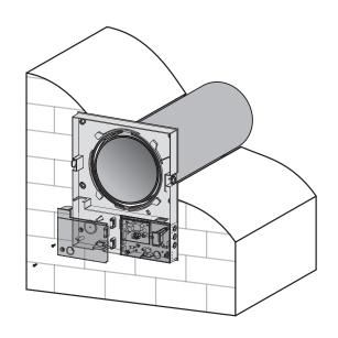
**6.** Insert the cartridge in the air duct as shown below. Be sure the pointer is directed upwards. Then fix the cable with a clamp and connect the socket connector to the control board.
