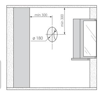
2. Insert the air duct in the wall using the supplied polystyrene wedges. The telescopic air duct end must protrude for the distance that enables installation of the outer ventilation hood.
