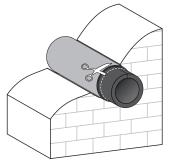
9. Insert the sound absorbing layer into the air duct. Roll the sound absorbing layer to match the air duct diameter with the protecting paper layer outside. Insert the roll in the air duct against stop against the cartridge. Make a mark at the end of the air duct, remove the material and cut the roll as marked. Insert the ready roll into the air duct.
