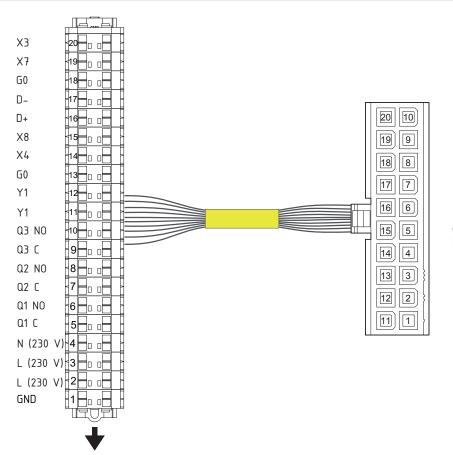
Matches contact in electrical compartment in system.
